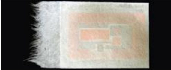
11. Encapsulated RFID tag from Washi Wrap as used at the Walker Art Center, Minneapolis. Copyright: Washi Wrap™ LLC
