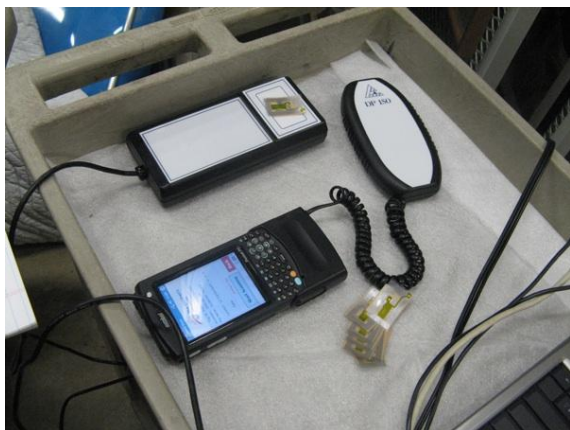
13. Tray with PocketPC running ARTifact TRAC software, RFID tags, and fixed and portable RFID reader/writers. Copyright: Children’s Museum of Indianapolis
