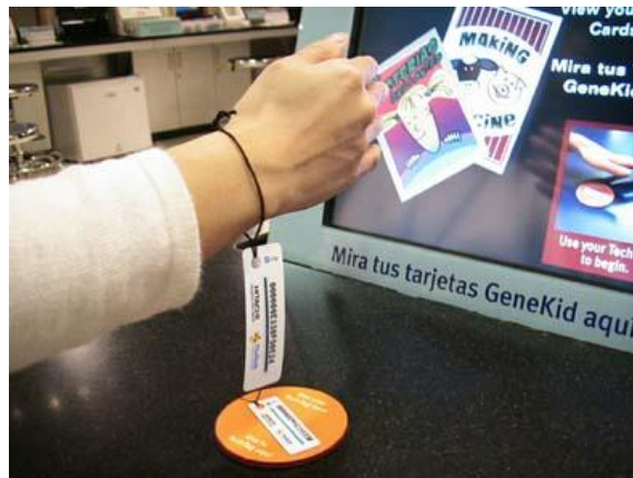
8. The TechTag at the Tech Museum activating an RFID reader embedded in the worktop. Copyright: Hitachi America Ltd
