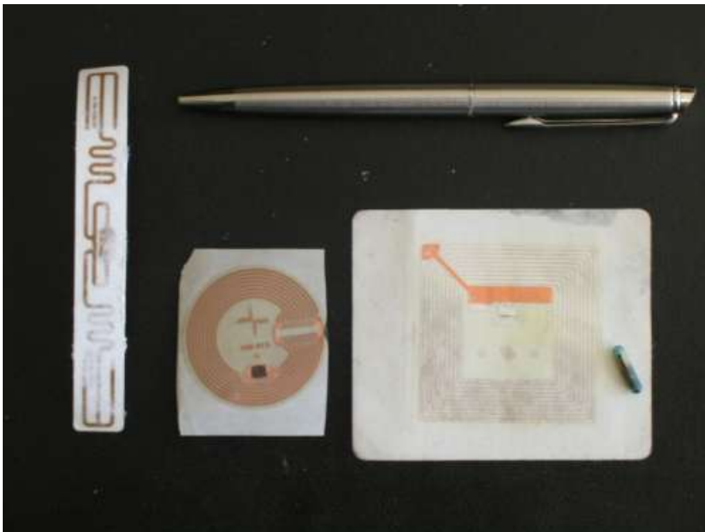
Figure 1. An example of RFID tags - 4 different types of tags with pen inserted for scale. Source: Doug Rogan, International Conservation Services
